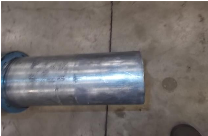
Coupling fit has visible damage
