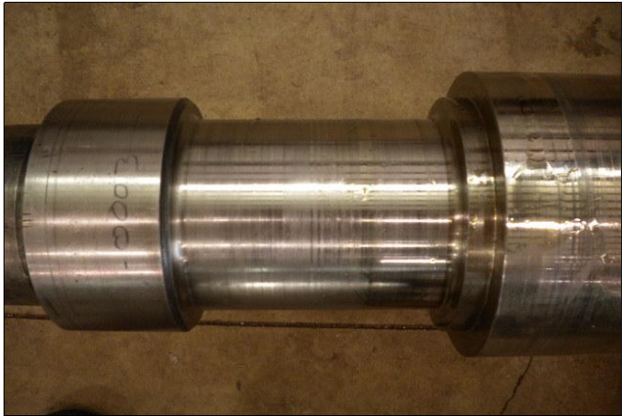
Inboard bearing journal is rough condition Probe areas are scratched
