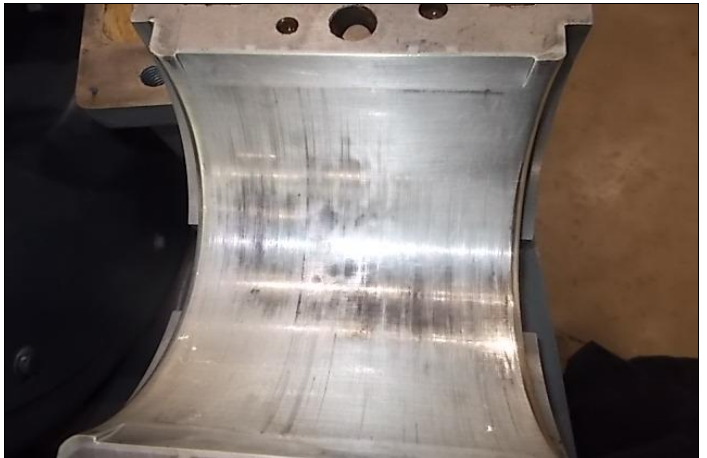
Bearings are oversized and have bad wear patterns
