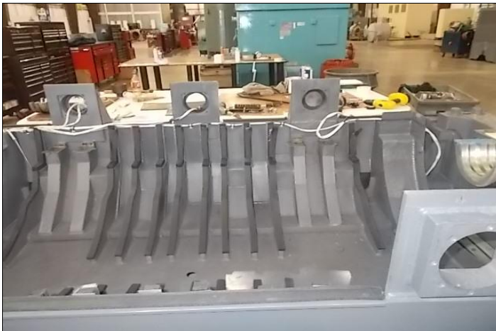
Bottom plate in frame is bent
